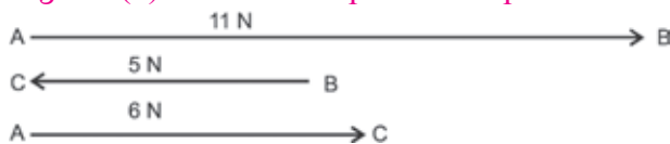
Fig 2.4 (b): Resultant of anti-parallel forces.
